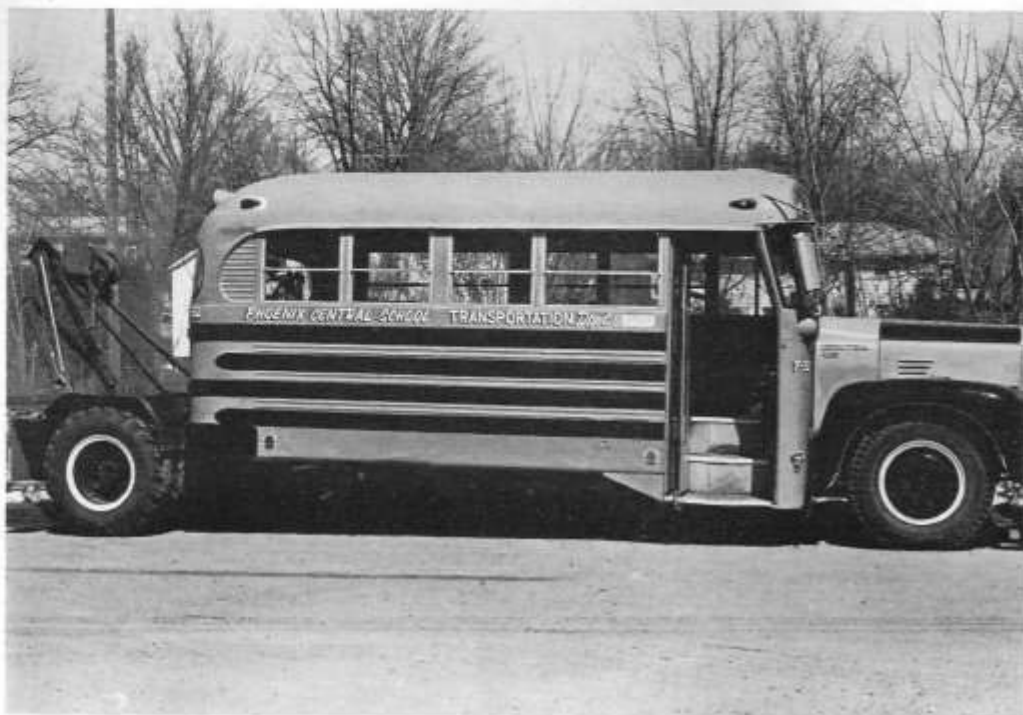
In conversion of coach (above) for maintenance duty with Phoenix, N.Y., school bus fleet, a saw removed back section and 12 feet from center of passenger compartment. New Jersey's 1803
