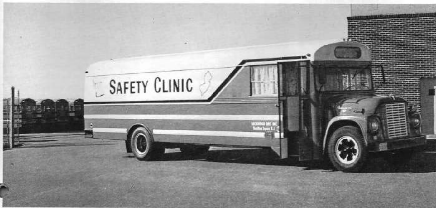
In conversion of coach (above) for maintenance duty with Phoenix, N.Y., school bus fleet, a saw removed back section and 12 feet from center of passenger compartment. New Jersey's 1803
